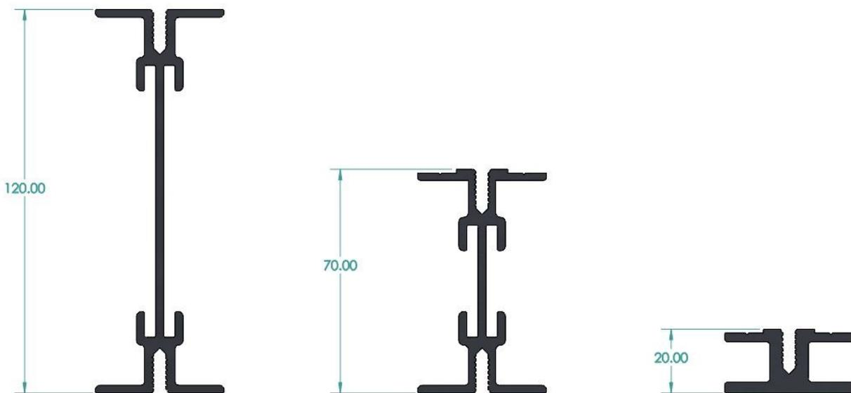
Aluminium Decking by Mextru is a complete decking system, with one of the most advanced, high strength substructure systems available on the market. The base structure is available in 3 standard heights to cover all your requirements, and all beam options are the same width, and use the same unique fixing system, which dramatically cuts down on-site installation time.
